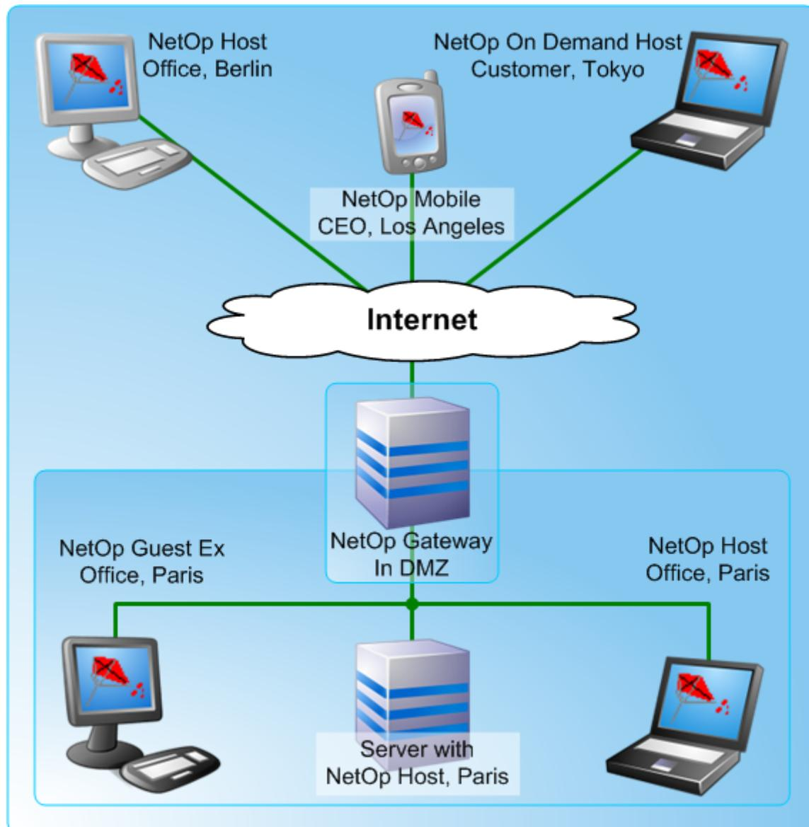
As the image shows, all traffic to and from the extended NetOp Guest has to pass the NetOp Gateway. The gateway is designed to act as a dedicated routing mechanism for
