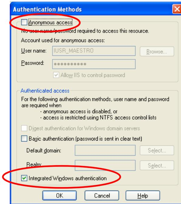
*Figure 9: Configure IIS to require user authentication.*
