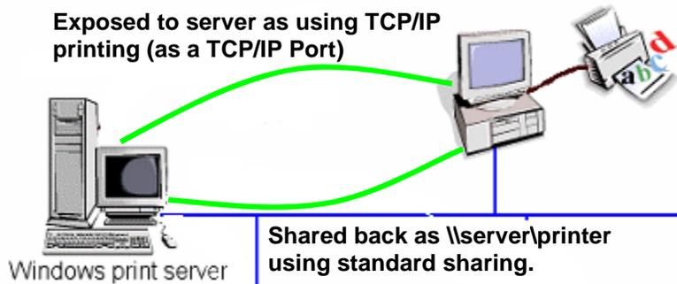
Figure 40—Desktop printers exposed using TCP/IP Printing and captured on server
