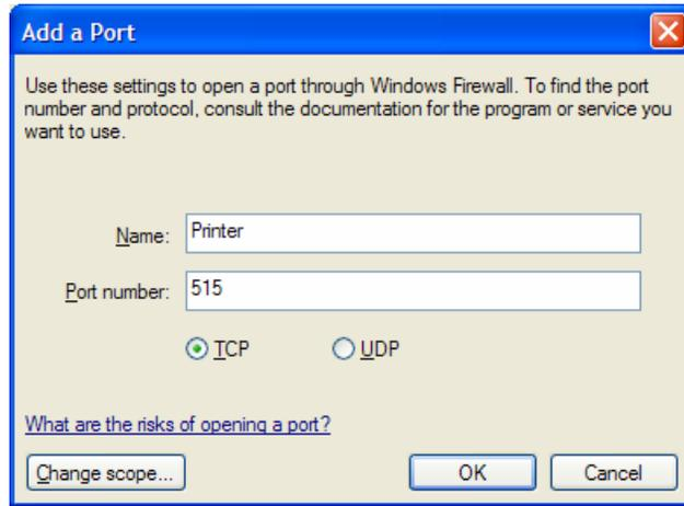
*Figure 44: Adding a firewall exception on port 515.*
