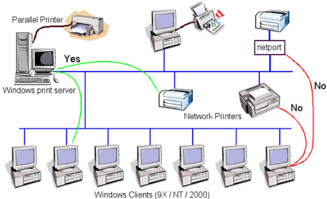
**Figure 1:** This network diagram includes clients, a print server, and printers.
