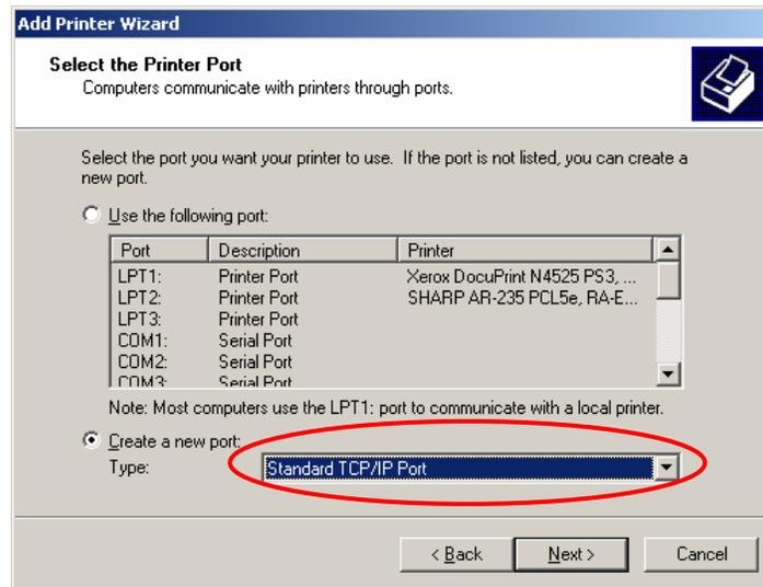
Figure 39 Select Standard TCP/IP Port
