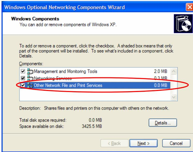
Figure 41 : Install TCP/IP print services
